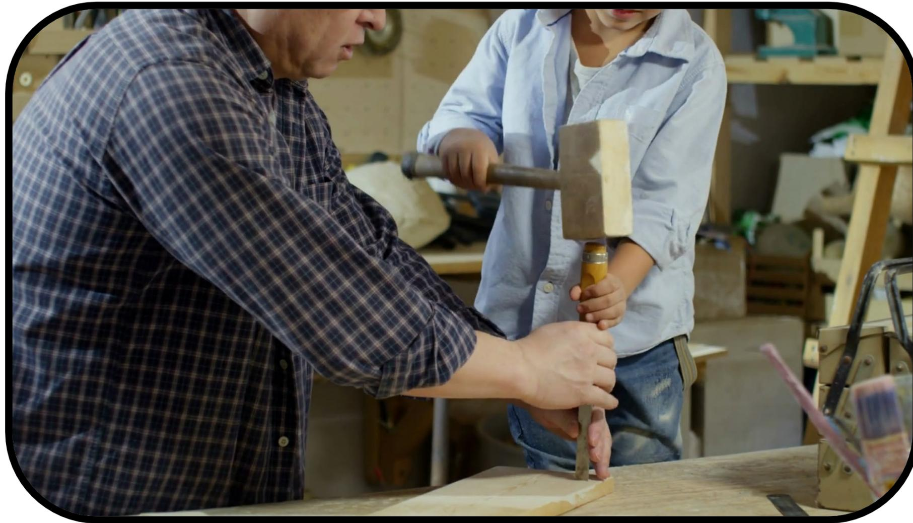
A **MALLET** is a hammer with a large wooden or rubber head.
